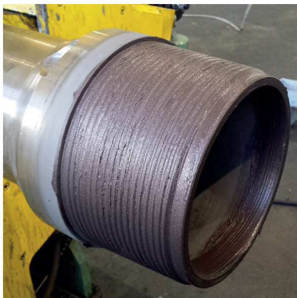
— Example of Swivel Joint Lower Body after correct dope application.
