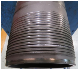
DOPELESS® 3.0/3.1 PIN AND BOX AFTER BREAK OUT
