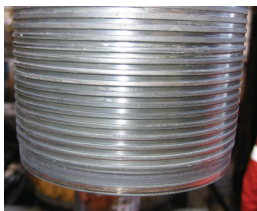
DOPELESS® PIN AND BOX AFTER BREAK OUT
